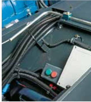
The external on/off switch enables quick service starts (an option).
